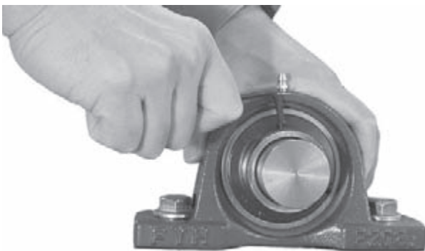
Fig. 14.5 Tightening of set screws
