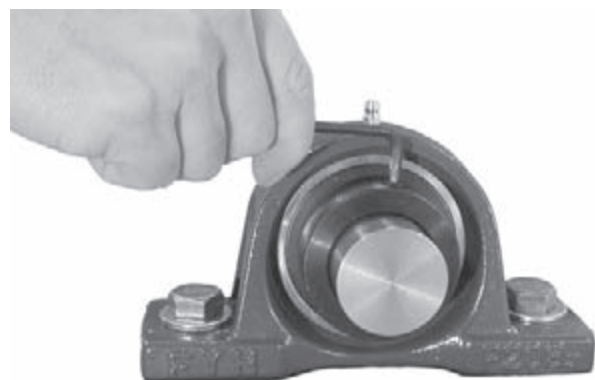
Fig. 14.10 Installing eccentric locking collar
