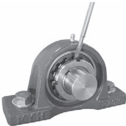
Fig. 14.8 Bending claw of washer (Locking locknut)
