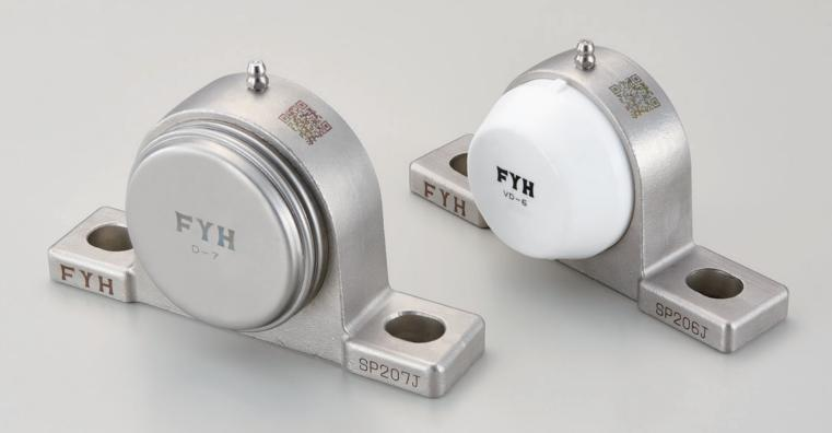
The redesigned shape and laser marked housings make the surface of our new stainless-steel housings smoother than ever. The flatter surface ensures there is no place for water to pool after washdown. The smooth housing and solid base reduce the risk of bacterial growth.
